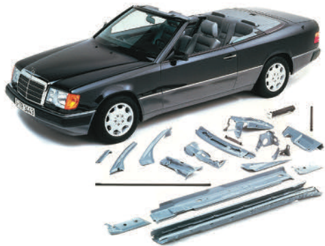
Cabriolet additionally installed body reinforcement parts
